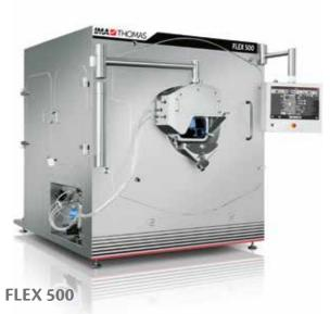
The FLEX 500 is a highly efficient tablet coating system designed for the special needs of the pharmaceutical industry, which features our patented exchangeable drum design. Standard configuration allows for all aqueous tablet coating processes including film, sugar, functional, and active multi-layer coatings. Optional features allow for organic solvent coating and various OEB containment levels for potent compound processing.
