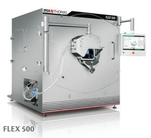
The FLEX 500 is a highly efficient tablet coating system designed for the special needs of the pharmaceutical industry, which features our patented exchangeable drum design. Standard configuration allows for all aqueous tablet coating processes including film, sugar, functional, and active multi-layer coatings. Optional features allow for organic solvent coating and various OEB containment levels for potent compound processing.
