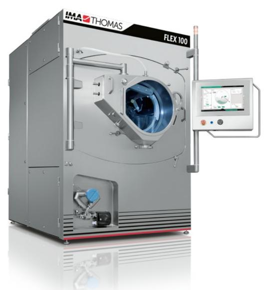
Designed to offer a wide variety of industry leading high-performance features, the Flex 100 features external gun positioning, auto unload, patented Thomas Spray Bar with Schlick patented ABC technology and 6 exchangeable drums allowing for capacity range of 2-125 Liters. The Flex 100 also comes with Wash-In-Place configurations and an optional containment version for use with highly potent products.
