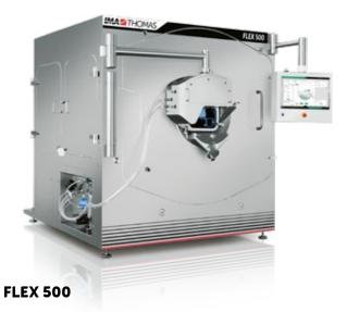
The FLEX 500 is a highly efficient tablet coating system designed for the special needs of the pharmaceutical industry, which features our patented exchangeable drum design. Machine capacity range of 40 – 920 Liters. Standard configuration allows for all aqueous tablet coating processes including film, sugar, functional, and active multi-layer coatings. Optional features allow for organic solvent coating and various OEB containment levels for potent compound processing.
